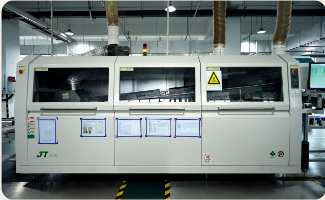
Three-proof coating line
